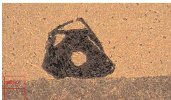
Fig. 2: Crystal growth at the phase interface of the air-sensitive elements Ca (bright) and Ce (gray). Light microscopical brightfield image of a microstructure.
