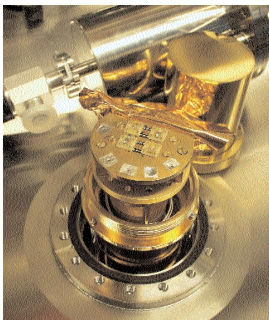
*Fig. 4: Cryostat for simultaneous measurement of the resistance of four samples. The device is mounted in an argon filled glove box and allows to load the samples without any contact to air.*
